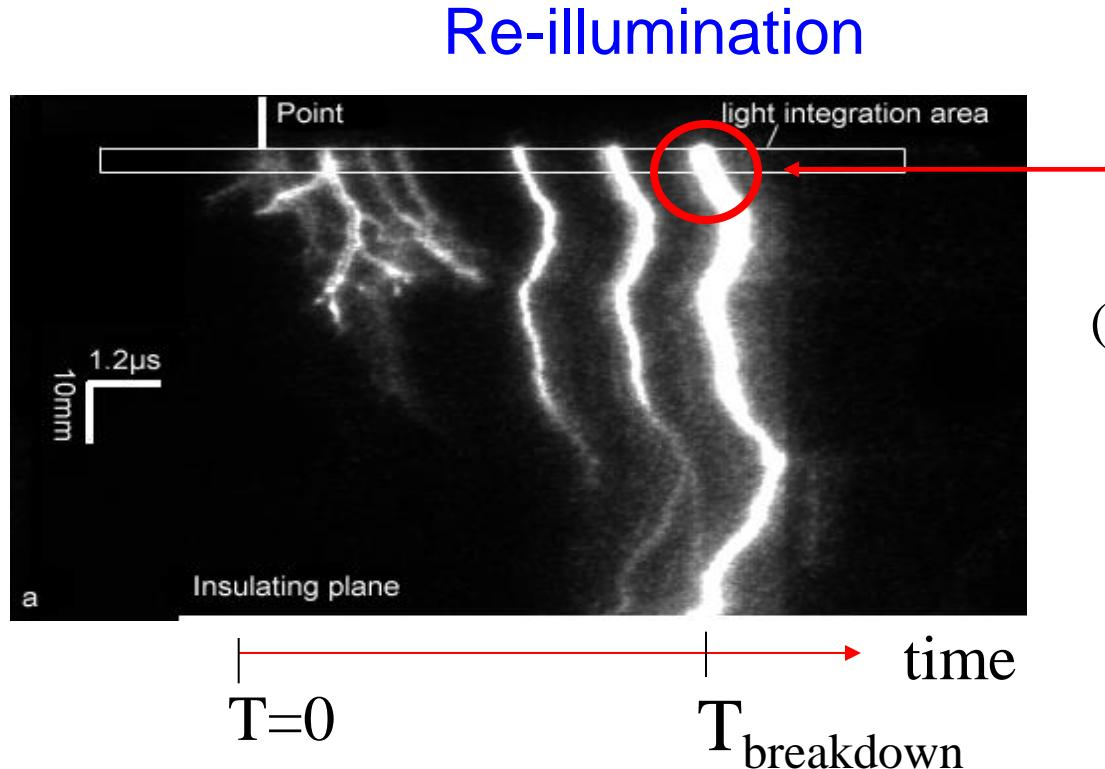
Light emitted by **one** positive streamer in LN<sub>2</sub> when it stops on the insulating plane
